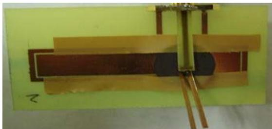
Figure 3. Jacket antenna clamped with a circular shaped ceramic material
