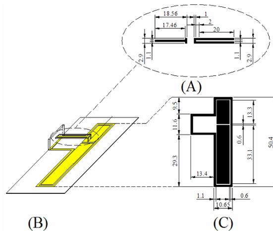
Figure 1. Schematic drawing of the design of the jacket antenna (unit:mm)
