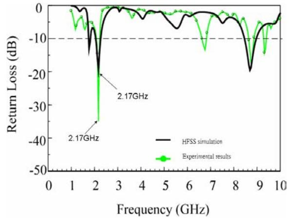
Figure 4. Return Loss of the jacket antenna clamping with a circular shaped ceramic material
