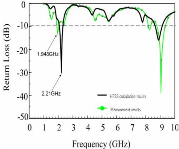
Figure 2. Experimental Return Loss and HFSS Simulation of the jacket antenna
