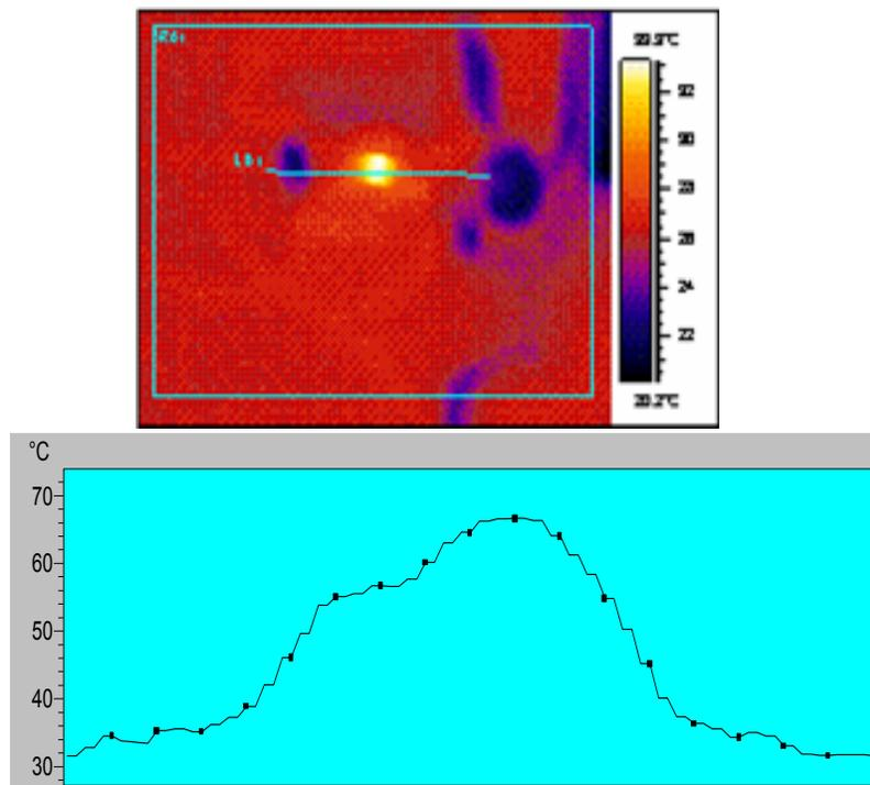
Figure 10. Temperature of arterial wall surface measured by thermal camera using a balloon catheter and diffuser fiber at 5W argon laser. The artery was perfused with whole blood circulating in an organ chamber.
