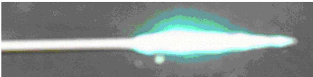
Figure 1. A standard angioplasty balloon catheter was used with a 300 µm optical fiber centered within the balloon. Argon ion laser irradiation can be seen as a bright light diffusing around the body of the inflated balloon.
