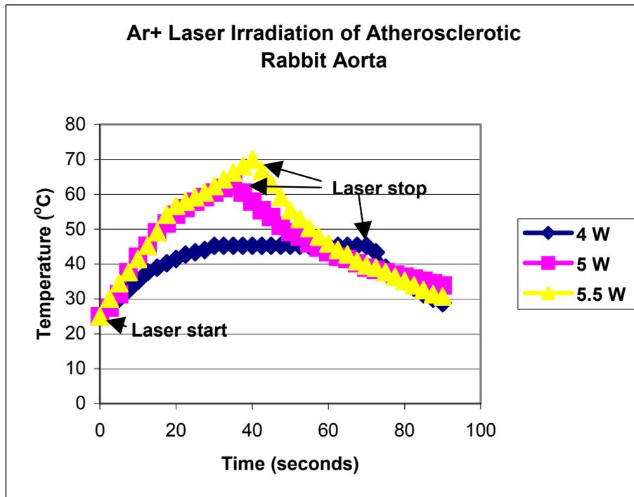
Figure 3. Temperature curves measured at the surface of the rabbit abdominal aorta during Ar<sup>+</sup> laser irradiation. These measurements were performed in a bath at 23°C.
