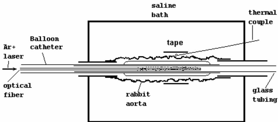
Figure 2. Sectional view of a single organ perfusion chamber. The balloon catheter is in the lumen of the rabbit artery. Thermal couples are placed on the surface to measure temperature and these are held in place using umbilical tape.
