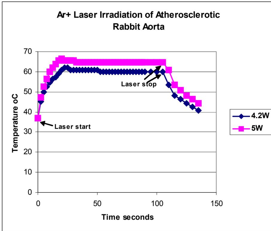
Figure 4. Temperature curves measured at the surface of the rabbit abdominal aorta during Ar<sup>+</sup> laser irradiation. These measurements were performed in a bath at 37°C to simulate the body temperature.
