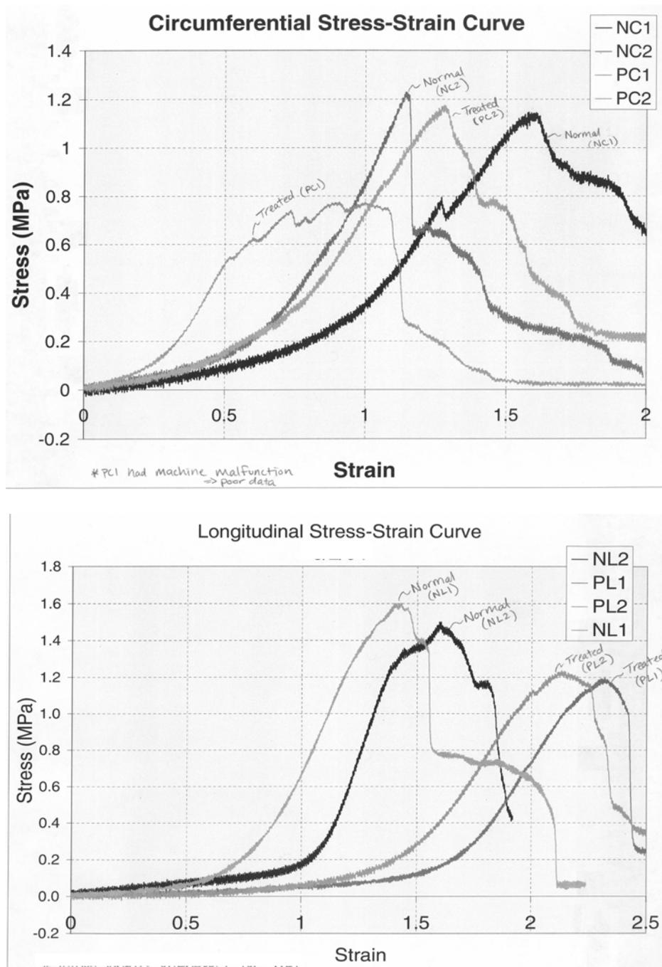
Figure 6. Stress-Strain measurement in the longitudinal direction (left graph) in the same artery above and at the site of laser treatment. Laser treatment demonstrates a shift of the curve to the right suggesting greater compliance. However, lowering of the peak stress suggests some reduction in tensile strength. The circumferential stress-strain curve (right graph) is probably similar but more data is needed to confirm the trend (the PC1 curve had a mechanical malfunction).
