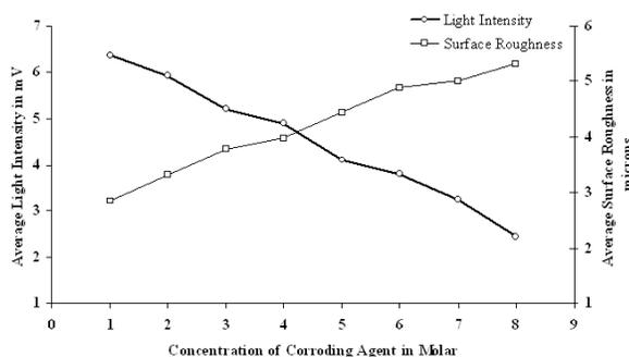
Figure 3. Comparison of average light intensity and average surface roughness for each molar concentration of corroding agent
