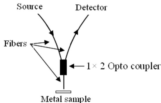
Figure 2. Schematic diagram of experimental setup
