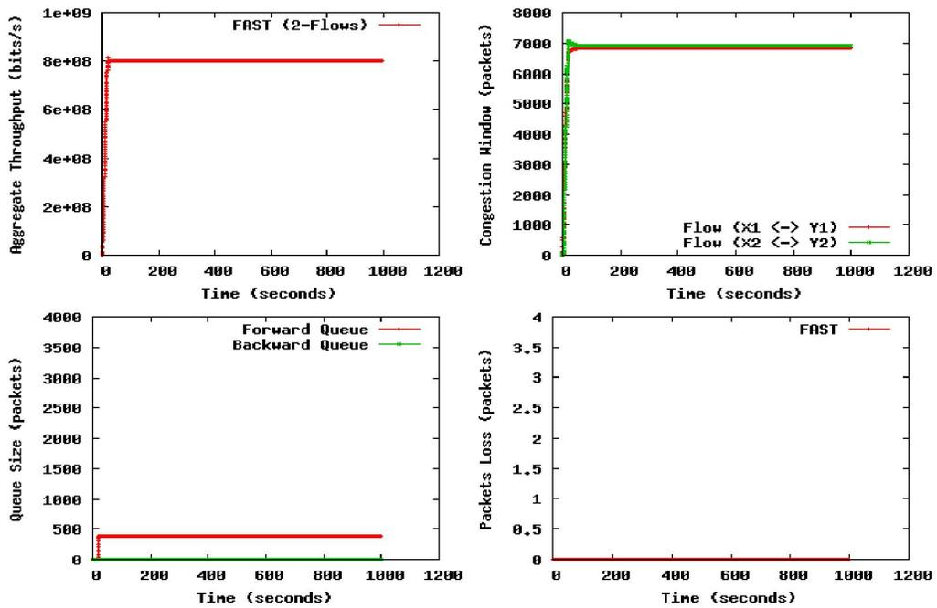
Fig. 3 FAST TCP's trajectories with 2-flows
