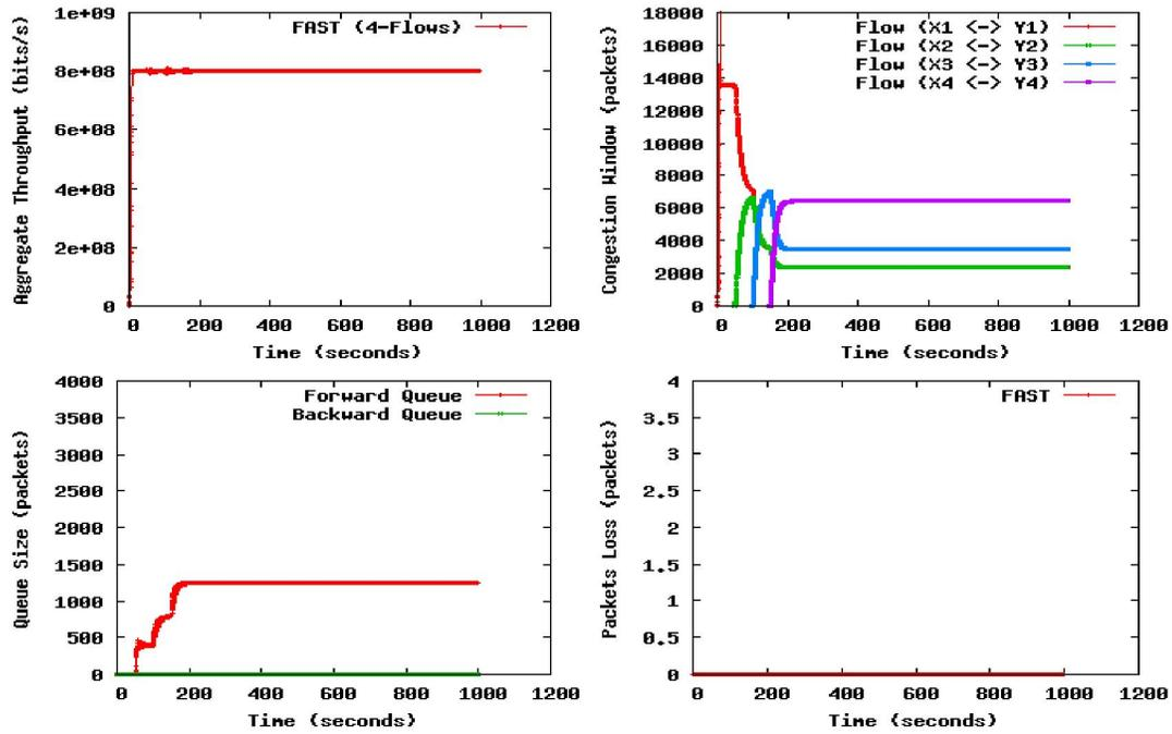
Fig. 5 FAST TCP's trajectories with 4-flows
