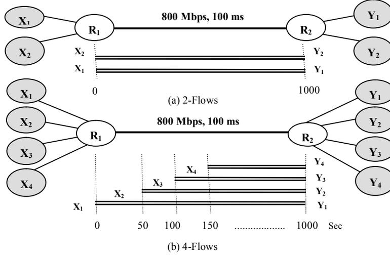
Fig.1 Network topology used in the simulations with active periods of the flows
