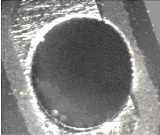
Figure 1. An Image of a Plated Through Hole on a Printed Circuit Board Showing Damage to the Conductor around the Hole
