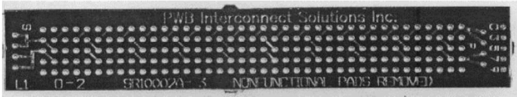
Figure 5. A Typical IST Test Coupon (adopted from PWB Interconnect Solutions, Inc)
