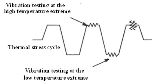
Figure 11. The Combined Temperature and Vibration Accelerated Life Test
