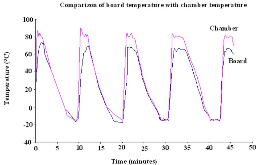
Figure 10. The Temperature Profile for the Board as Compared with the Chamber Showing a Lag in the Board following the Temperature of the Chamber
