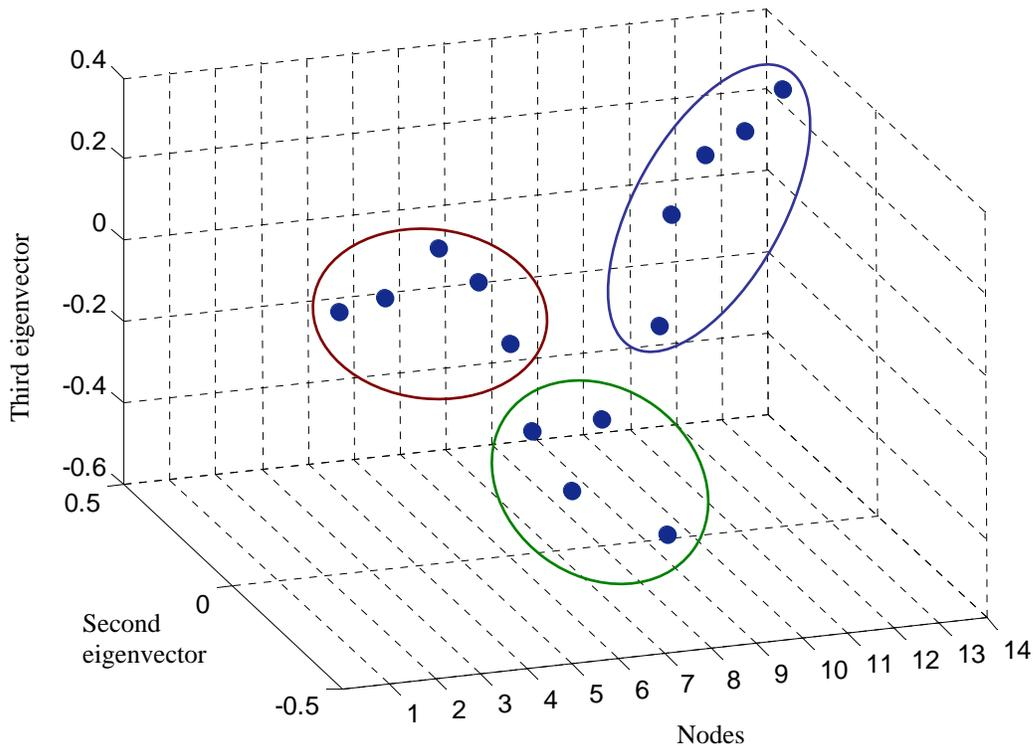
Figure 6 The second and third eigenvectors with respect to the nodes and the three partitions of the power system based on the eigenvectors of the Laplacian of the graph
