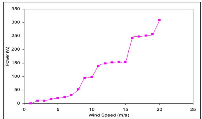
Figure 12. Alternating current (a.c.) Power Curve at sea level air density, 1.225kg/m<sup>3</sup>
