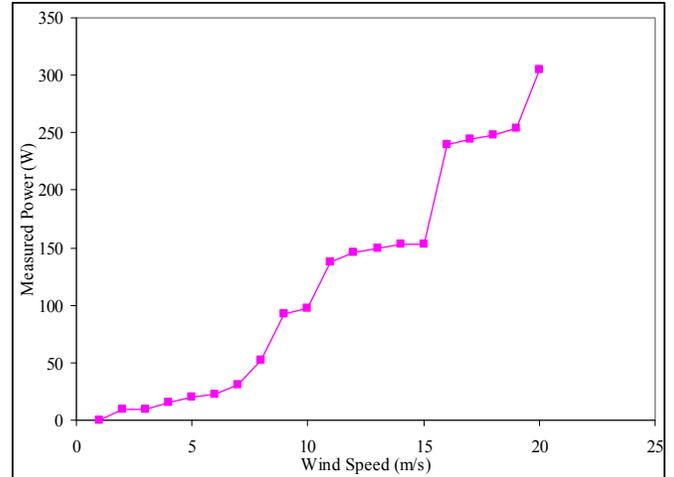
Figure 11. Alternating current (a.c.) Power Curve at site average air density, 1.21kg/m<sup>3</sup>
