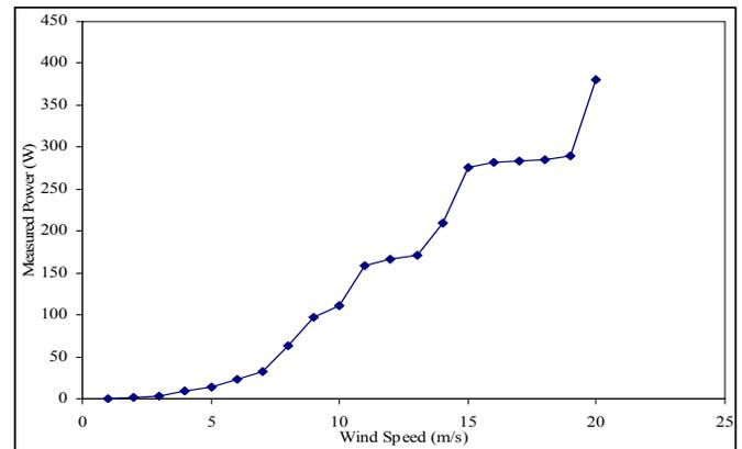
Figure 9. Direct current (d.c.) Power Curve at site average air density, 1.21kg/m<sup>3</sup>
