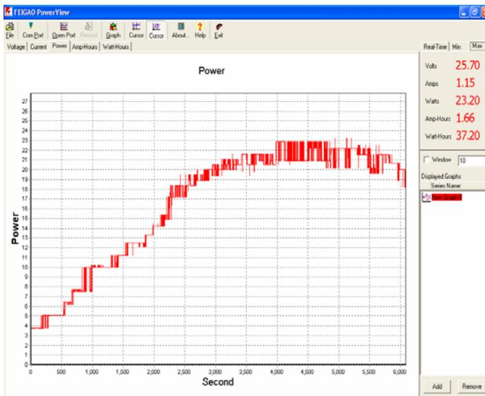
Figure 8. Test Turbine Power measurement using Power Analyzer
