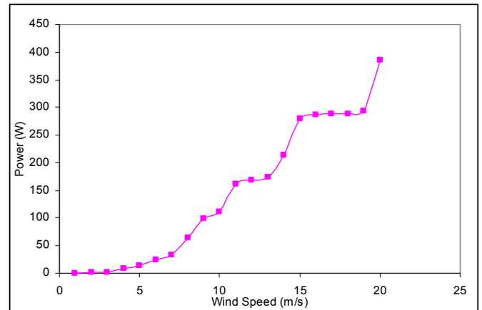
Figure 10. Direct current (d.c.) Power Curve at sea level air density, 1.225kg/m<sup>3</sup>
