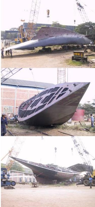
Figure. 5 Overturning Process
