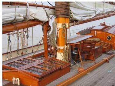
Figure.9 Hatch, Mast and Boom
