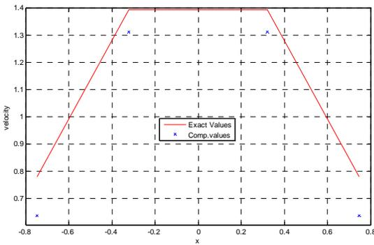
Figure 3: Comparison of computed and analytical velocity distributions over the surface of a sphere using 24 boundary elements
