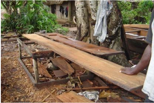
Plate 1.1: Planks placed on attendant for framing before it is used in canoe construction at Epe.
