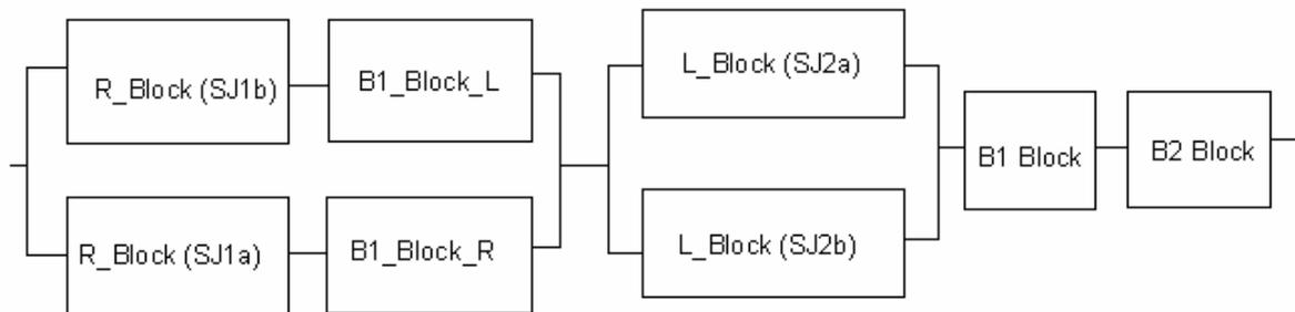
Fig. 5. The reliability block diagram of fuze electronics
