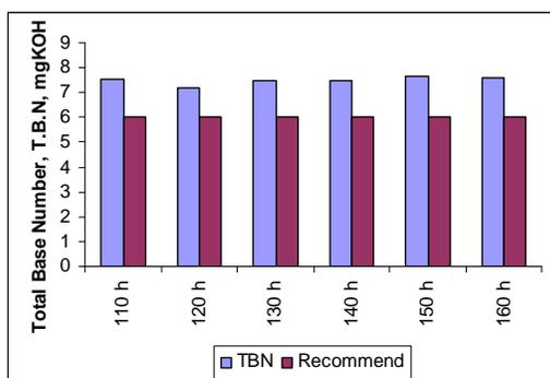
Fig 6: TBN changes during the different running hours
