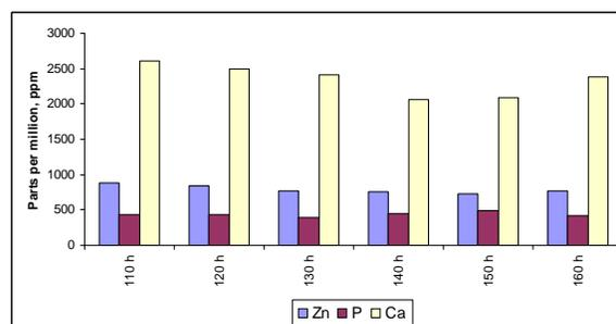
Fig 2: Result of additive materials analysis during different running hours
