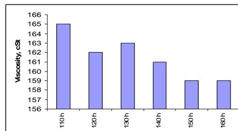
Fig 5: Viscosity analysis results during different running hours
