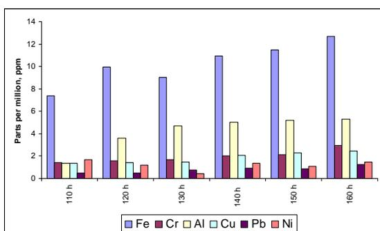
Fig 1: Wear debris analysis results during different running hours
