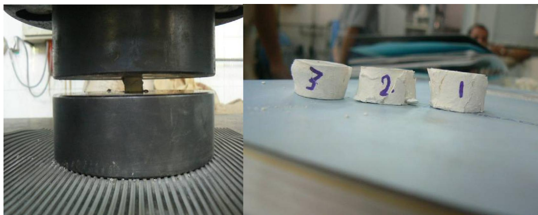
Figure (3): Failure patterns of some of the tested specimens.
