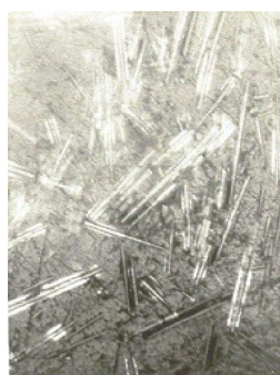
A) 17% fibre, L/D=50 , 500x b) 50 % fibre, L/D=50 , 500x C) 17% fibre, L/D=1 , 500x D) 50 % fibre, L/D=1 , 500x Fig (4) the fibre impeded into the matrix before laser irradiation at 500x and at different percentages of fibres.
