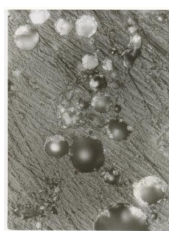
A) 17% fibre, L/D=50 , 500x b) 50 % fibre, L/D=50 , 500x C) 17% fibre, L/D=1 , 500x D) 50 % fibre, L/D=1 , 500x Fig (4) the fibre impeded into the matrix before laser irradiation at 500x and at different percentages of fibres.
