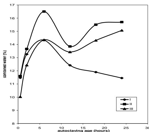
Fig.(4): Combined water contents of Mixes I, II and III at various autoclaving ages.
