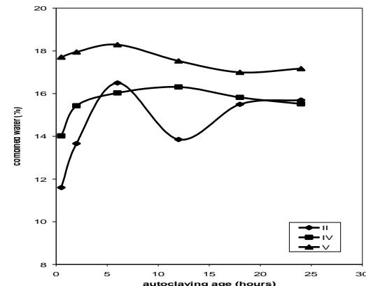
Fig.(5): Combined water contents of Mixes II, IV and V at various autoclaving ages.
