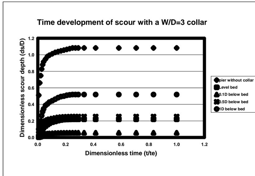
Figure 8. Time development of scour for different elevations
