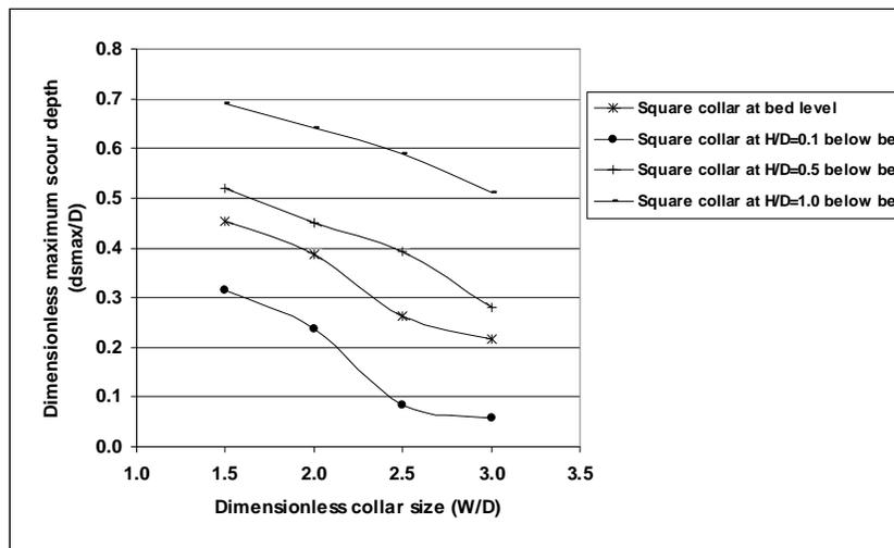
Figure 7. Maximum scour depth for different collar sizes
