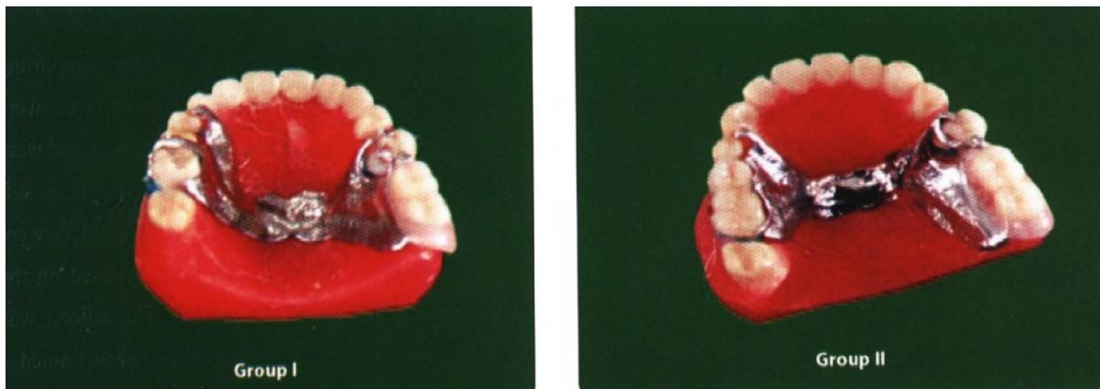
**Fig. (3.4) Strain gauges cemented in their sites in the prepared acrylic casts for both groups.**
