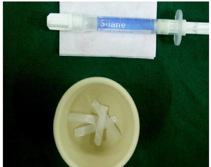
**Fig.4: Glass fibers soaked in silane coupling agent**
