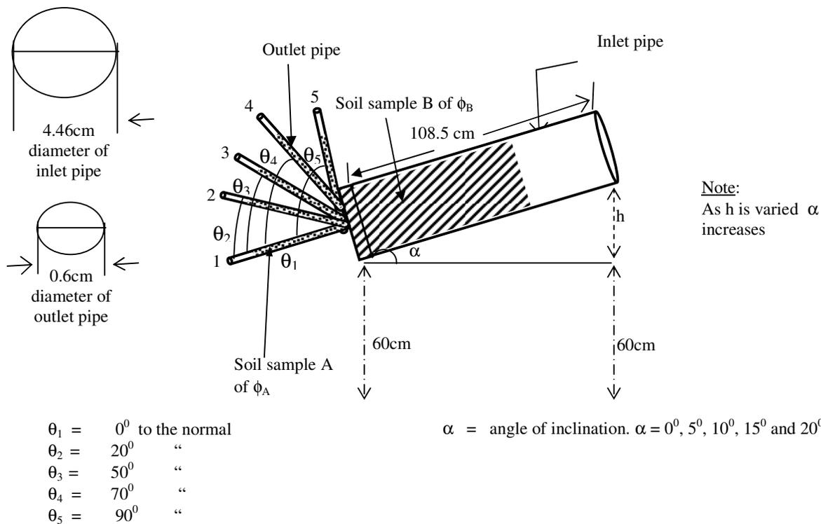
Figure.2: Schematic Diagram of set-up to determine volume flux at different outlet angles.
