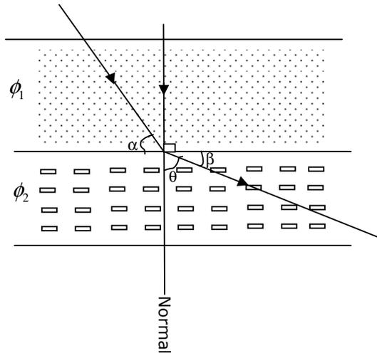
Figure 1: Schematic diagram to show the relationship between refracted angle and deflection angle.
