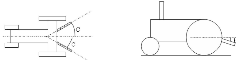
Figure2- position of forces in top arm- Left: axis force and its angle with horizontal plane (a) –right: analyzing of axis force to tension and vertical components
