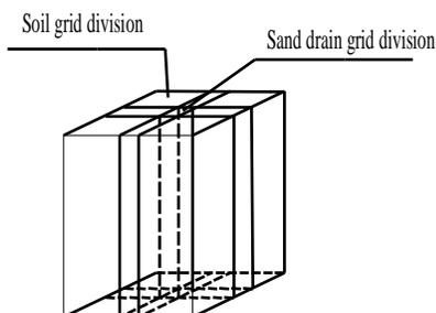
Figure 2a Conventional sand drain element partition
