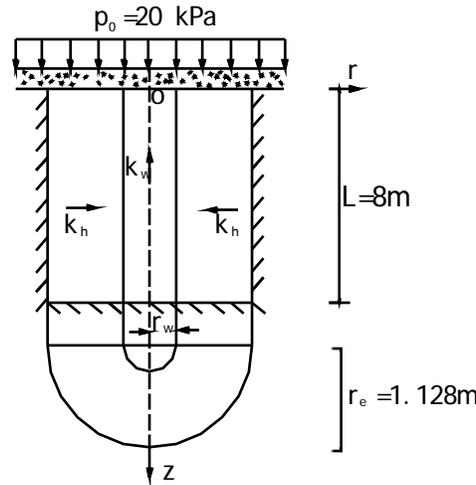
Figure 4 the sketch of single sand drain
