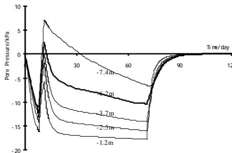
Figure 9a General Element pore water pressure
