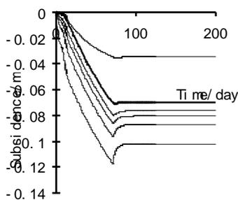
Figure 8b. Sand Drain Element stratified settlement
