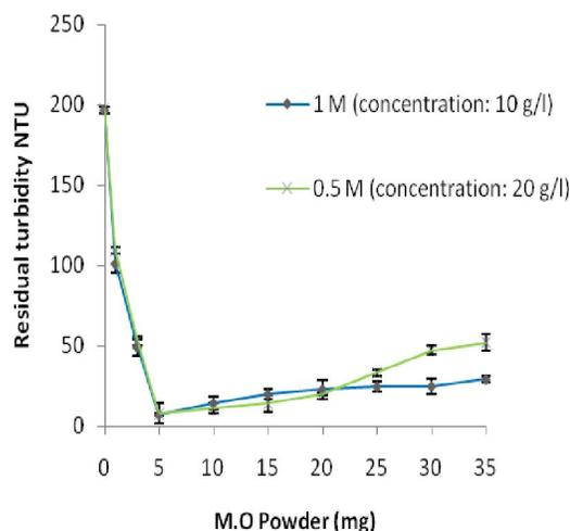
Figure 5: Average residual turbidity after coagulation with MOC-SC-SD solutions
