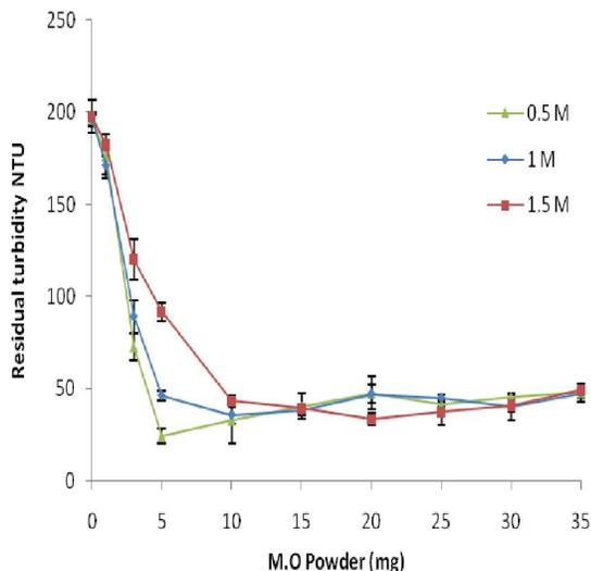
Figure 4: Average residual turbidity after coagulation with the MOC-SC solution of 200 g/l concentration
