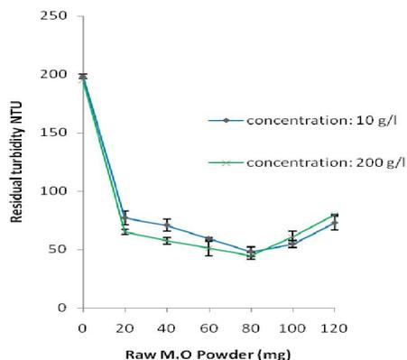
Figure 2: Average residual turbidity after coagulation with the MOC-DW solution of 10 g/l and 200 concentrations
