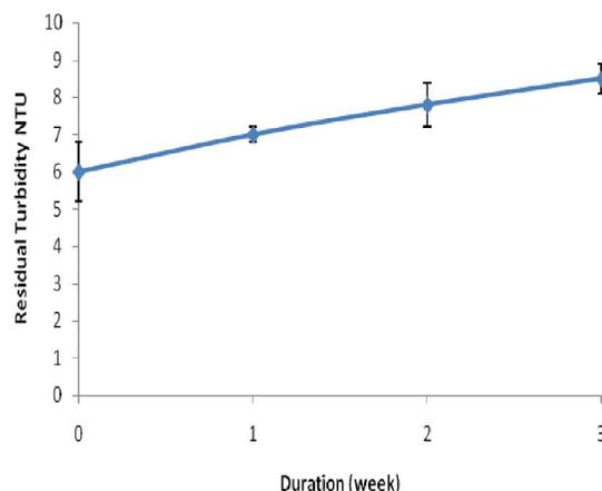
Figure 7: Effect of storage duration of M.O. powder on residual turbidity
