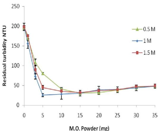
Figure 3: Average residual turbidity after coagulation with the MOC-SC solution of 10 g/l concentration
