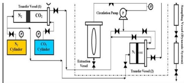
Fig 4: Schematic diagram of the Supercritical Fluid Extraction System (SCFE) for Extraction of oil from canola seed with supercritical carbon dioxide.
