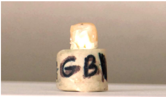
Figure 1: A representative longitudinal fracture for one specimen.
