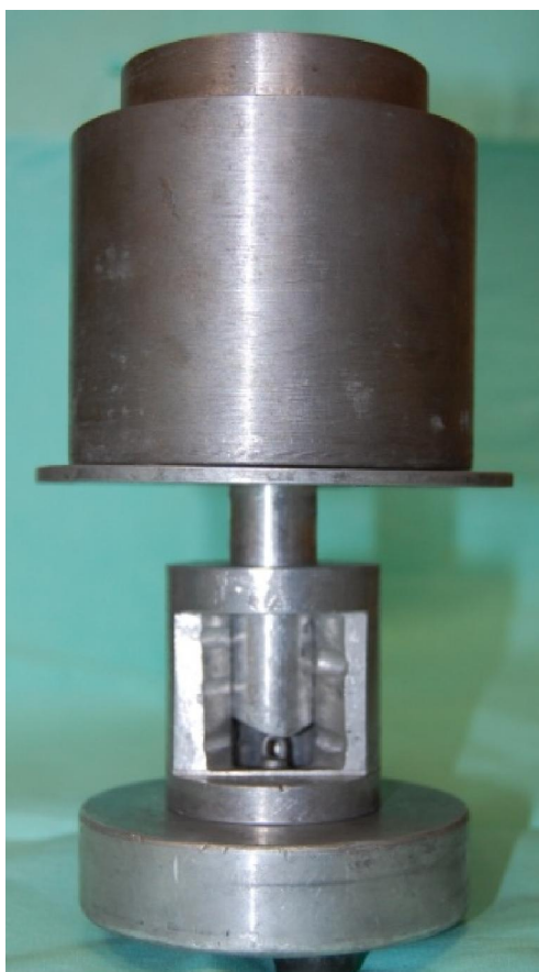
Figure 2: Metal coping sample within the cementing device
