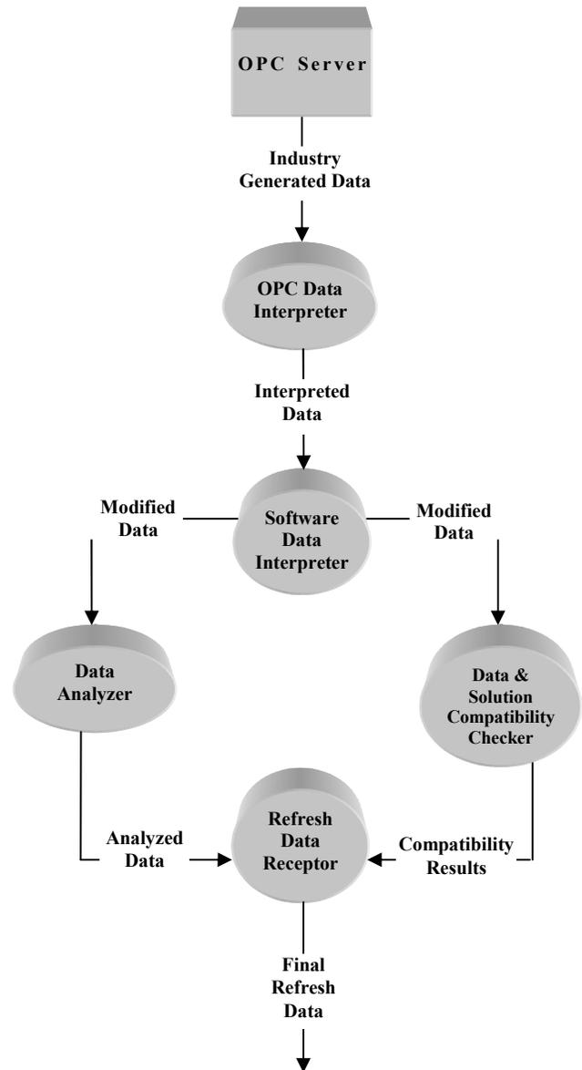
Figure 3. Second level DFD of the system
