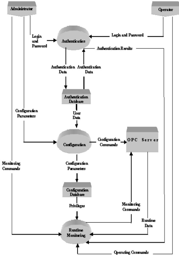
Figure 2. First level DFD of the system
