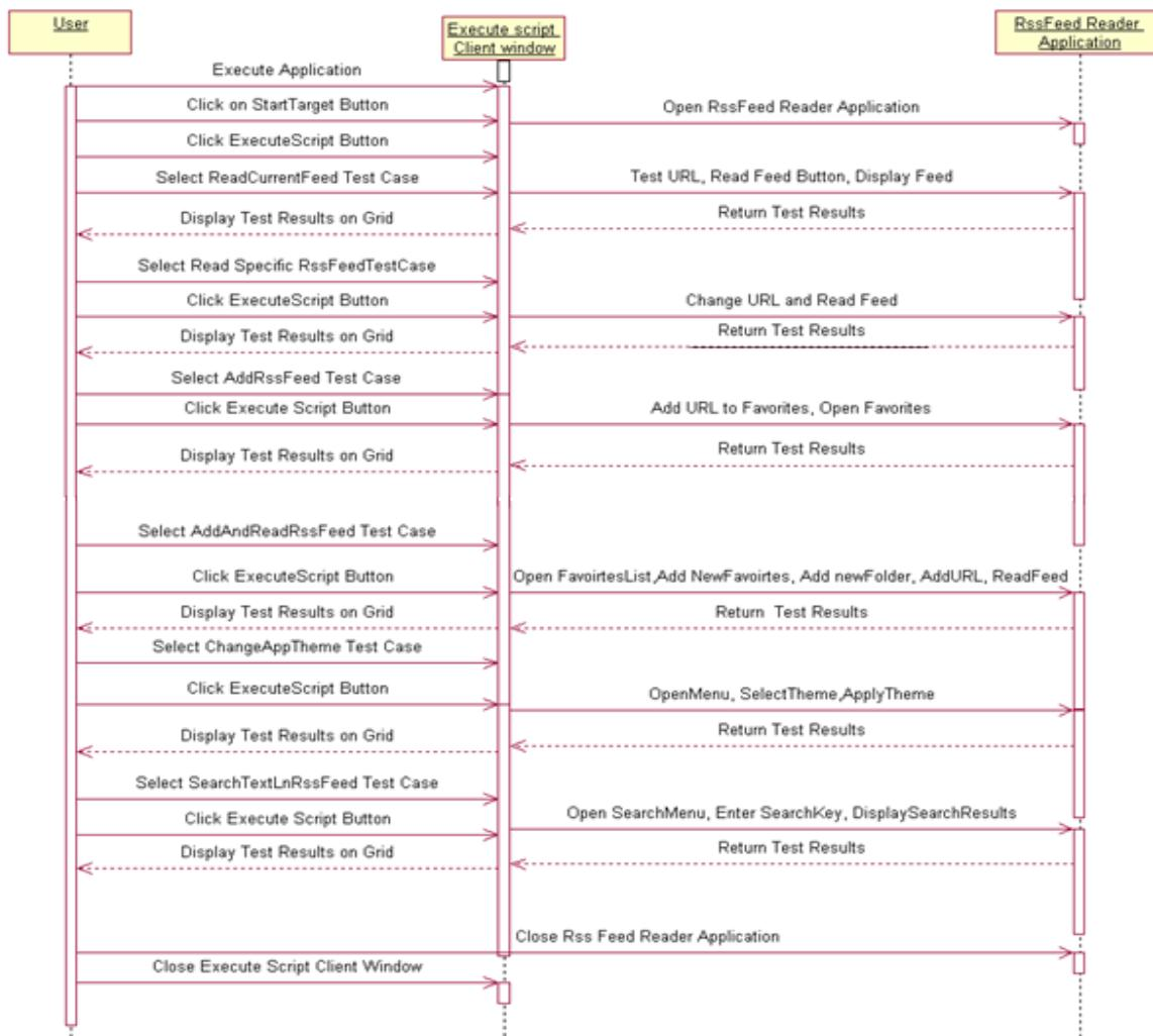
Figure 2: System sequence diagram of proposed framework
