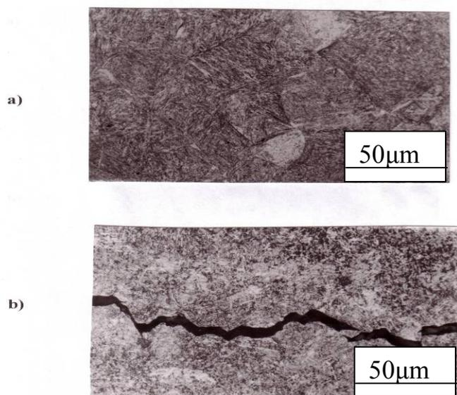
**Fig. 5** Microstructure at the HAZ of the base metal a) Crack free specimen,
