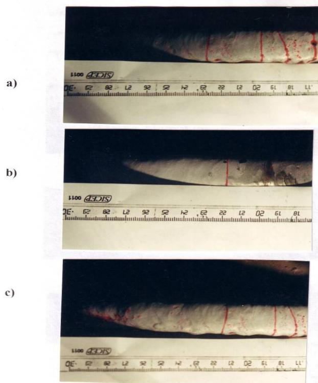
**Fig. 2 Transverse surface cracks by dye penetrant test**
