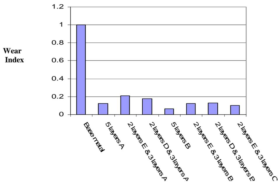
**Fig. 9** Wear index for base metal and hardfacing layers
