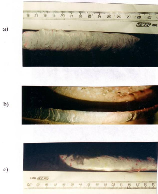
**Fig 3** weld beads free from cracks as detected by dye penetrant test
