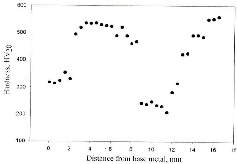
**Fig. 8** Hardness distribution along the base metal, HAZ and hardfacing material using electrode E and three layer of electrode A.
