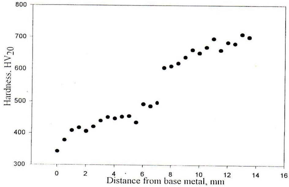
**Fig. 7** Hardness distribution along the base metal, HAZ and hardfacing material using electrode A
