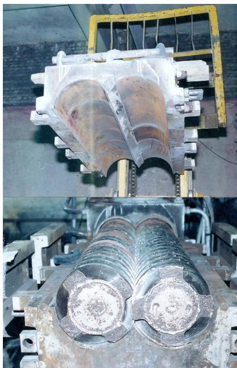
**Fig. 1 Complete structure of the extruder and the location of the screw conveyor**
