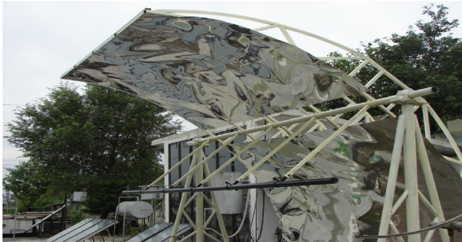
Fig. 4 Frame structure of parabolic trough collector design and developed by researchers
