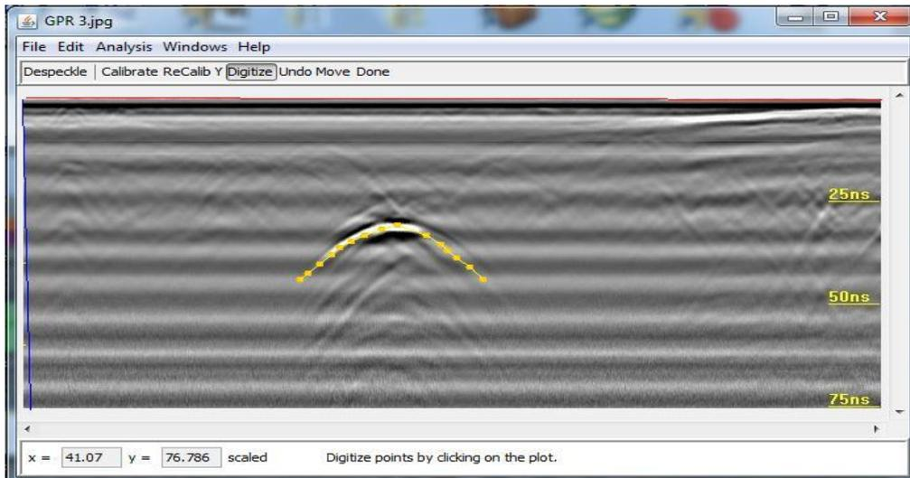
Fig. 3, digitized radar scan
