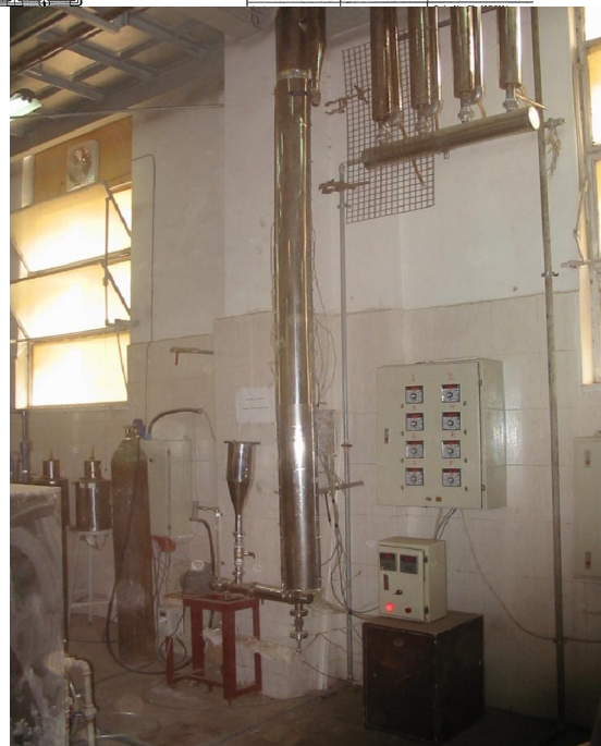
1-cyclone cooler/condenser, 2- reactor/ cyclone connection, 3-cyclone, 4, 5, 6-1 st , 2 nd , 3 rd 4 th cooler/condensers, 7, 8-condensate collectors and accessories, 9- reactor, 12-sleeve, 14-feeding hopper, 17-screw,
