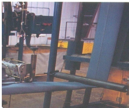
Fig. 5. Woven fiber glass bags are sewn with three needle chain stitch in vertical seam
