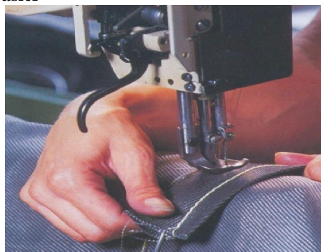
Fig. 4 Anti-collapse rings into filter Bags using lock stitching
