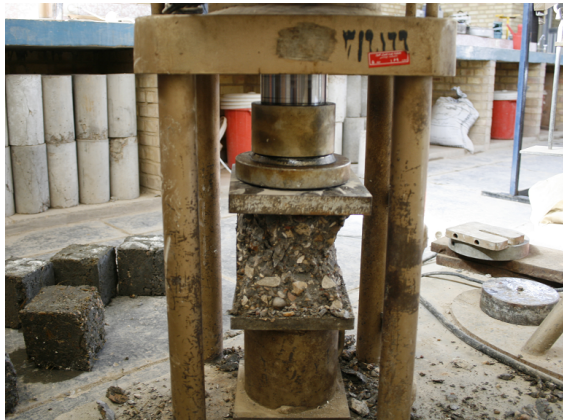
Figure 4. Fracture of the cubic sample of LWC
