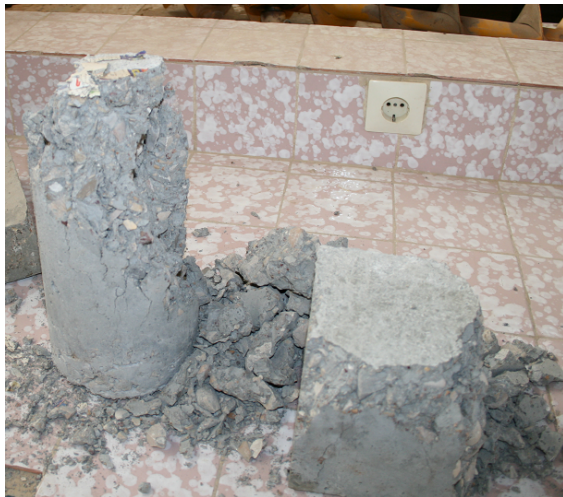
Figure 5. Different mode of the fracture of the cylindrical and cubic samples of LWC including Bagasse
