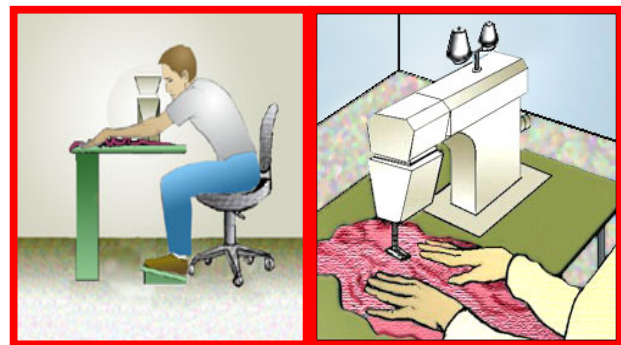
Figure (7): illustrates the effect of the design of inclination angles of sewing table and its sharp edges on hands and arms pain
