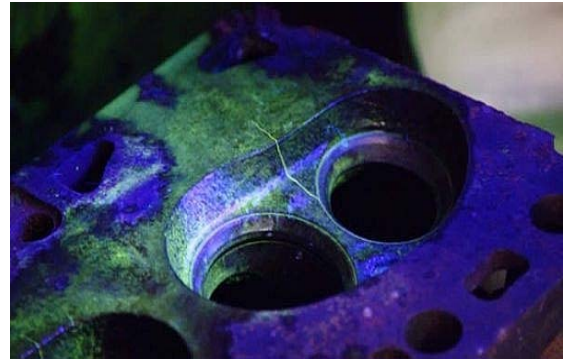
Fig. 1 Crack as detected by fluorescent magnetic particle test
