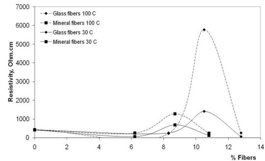
Fig. (8): Effect of volume percent fibers on AC resistivity of samples at 1 MHz and 30°C
