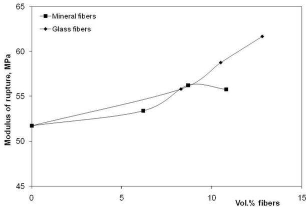
Fig. (6): Effect of volume percent fibers on flexural strength
