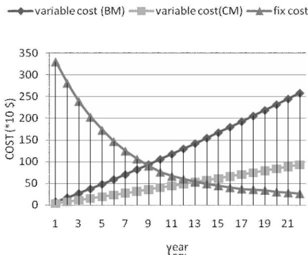
Figure1. Repair and maintenance cost of tractors BM and CM method in Iran
