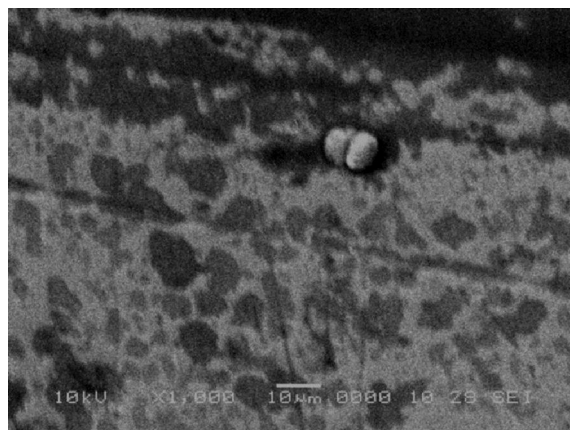
Fig. (9a).SEM of nickel deposited from bath containing 0.2 mol/l \text{NiSO}_4 \cdot 6\text{H}_2\text{O} and 0.2 mol/l \text{C}_6\text{H}_{11}\text{NaO}_7 with 0.4 mol/l boric acid and 0.4 mol/l ammonium sulfate at pH 8, time 20 min and temperature 25^\circ\text{C} , current density 2.5 \text{ A/dm}^2 .
