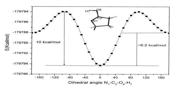
Fig.1: The energy profile for the rotation of the O-H group in 2-pyrrolidinol by B3LYP/6- 311G(d,p) basis set.
