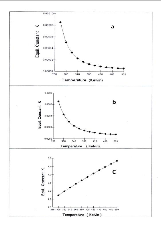
Fig.6: Variation of equilibrium Constant (K) with temperature for the conversion process of (a) monomer 2-pyrrolidinone to cyclic trimer; (b) monomer 2-pyrrolidinone to open trimer; (c) cyclic trimer to open trimer.
