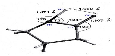
Fig.2: The characteristic structural parameters of the transition state of ketoenol conversion.
