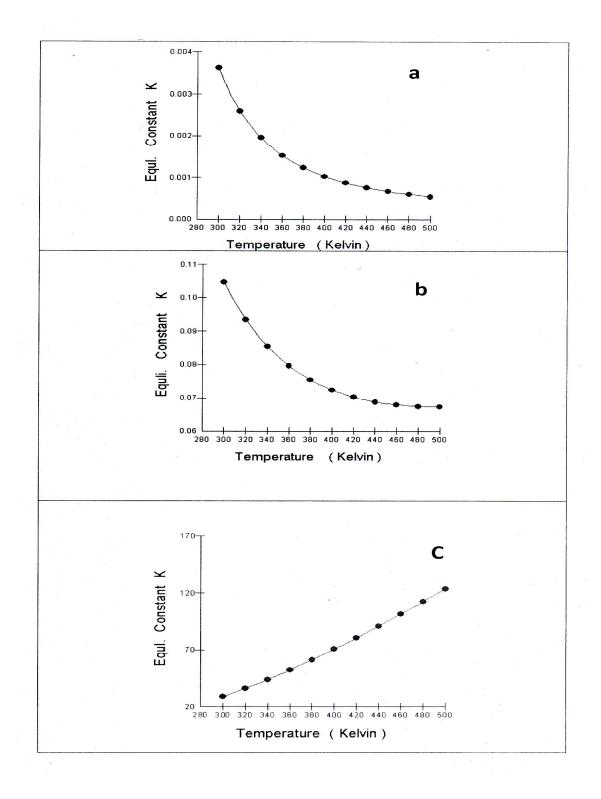
Fig.5: Variation of equilibrium Constant (K) with temperature for the conversion process of (a) monomer 2-pyrrolidinone to cyclic dimer; (b) monomer 2-pyrrolidinone to open dimer; (c) cyclic dimer to open dimer.
