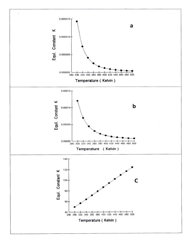
Fig.7: Variation of equilibrium Constant (K) with temperature for the conversion process of (a) monomer 2-pyrrolidinone to cyclic tetramer; (b) monomer 2-pyrrolidinone to open tetramer; (c) cyclic tetramer to open tetramer.
