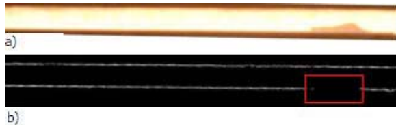
Fig 10a) Edge of tile that has crack, Fig 10b) edge crack is detected after applying algorithm
