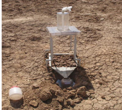
Fig 2.rainfall simulator that was used on site to evaluate the relative erodibility of formations.
