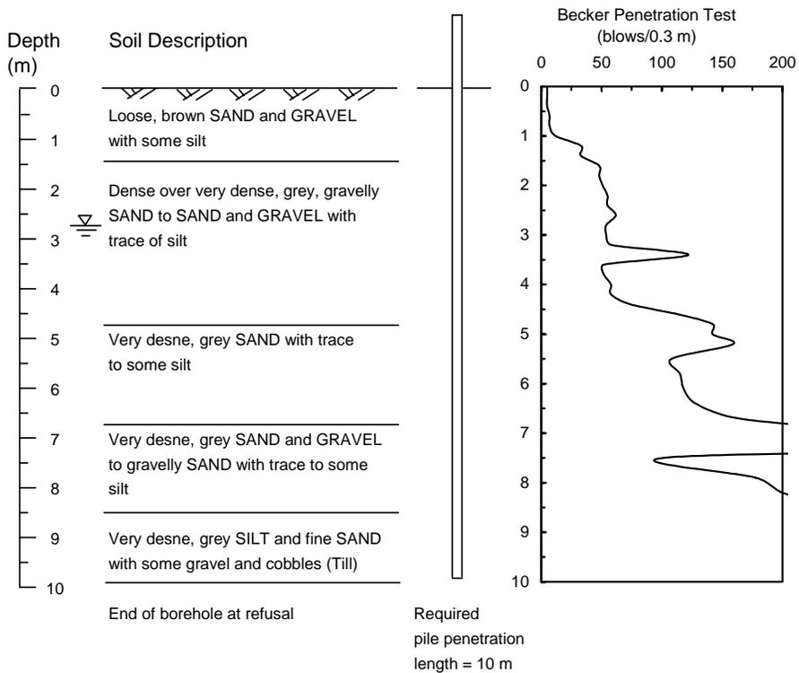
**Fig.7 Soil conditions and Becker Penetration Test results for Case History 2**
