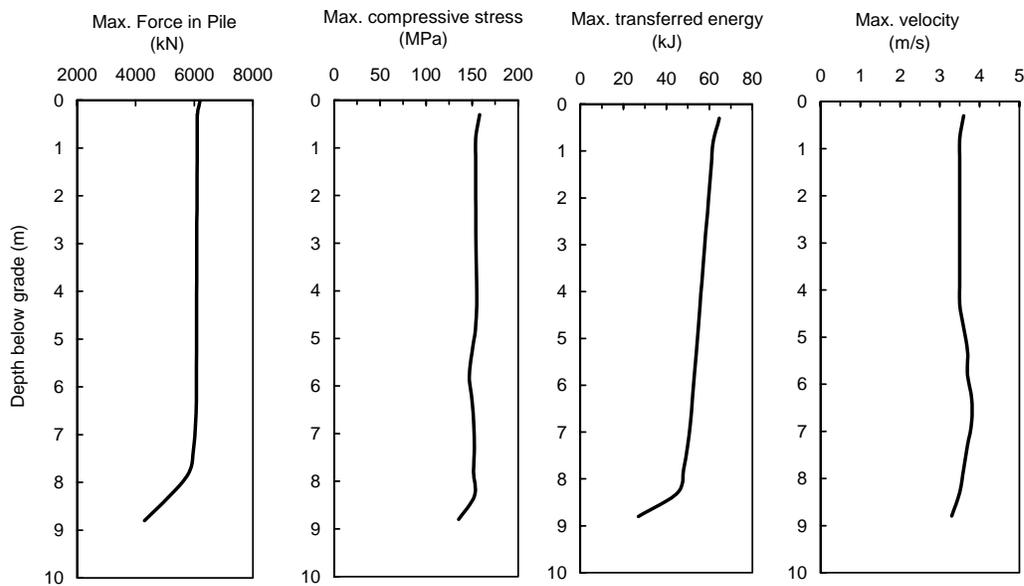
**Fig. 5 Maximum force, compressive stress, transferred energy and velocity along the length of Pile No. 1 derived from CAPWAP results (Case History 1).**
