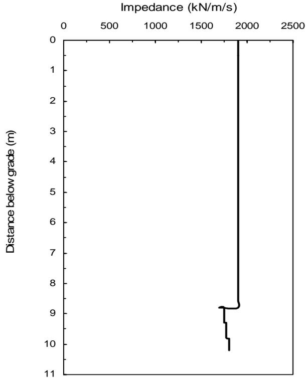
**Fig. 6 Impedance profile for Pile 2 indicating damage within the lower 1.5 m (Case History 1)**
