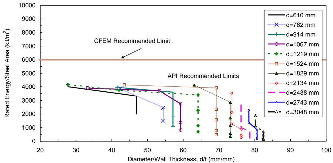
**Fig.1. The ratio between pile diameter to wall thickness, d/t, versus rated hammer energy/steel area (based on recommendations of API, 2007 and Canadian Foundation Engineering Manual (CFEM), 2006)**
