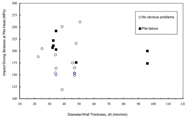
**Fig. 11. Data presentation of case studies for d/t ratio versus impact driving stresses at pile head ( $F_y = 300$  MPa)**
