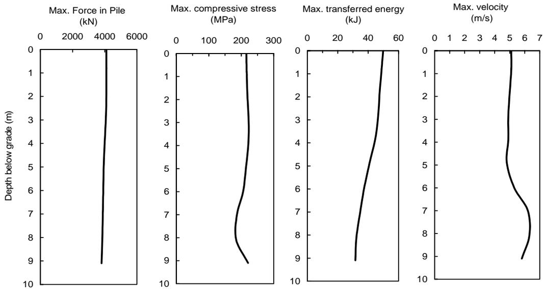
**Fig. 8 Maximum Force, compressive stress, transferred energy and velocity along pile length derived from CAPWAP results (Case History 2)**
