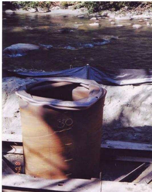
**Fig. 3. Pile head failure (d=1219 mm, t=12.7 mm), driven by D60-62 diesel hammer (Case History 1)**
