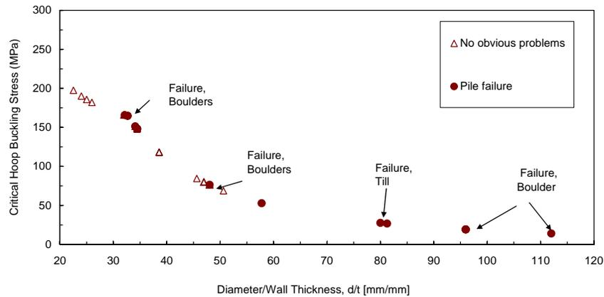
**Fig. 12. Data presentation of case studies for d/t ratio versus critical hoop buckling stresses ( $F_y = 300$  MPa)**
