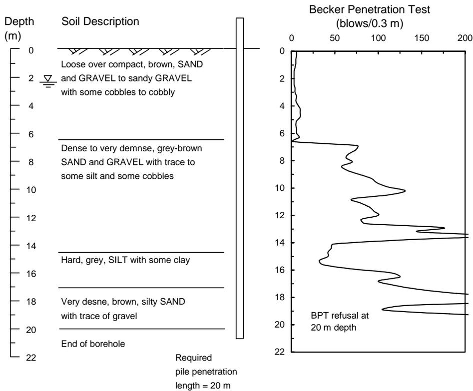
**Fig.9 Soil conditions and Becker Penetration Test results for Case History 3**
