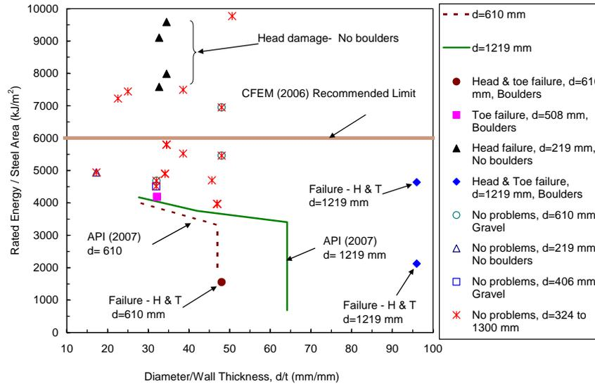
**Fig. 10. Data presentation of case studies for d/t ratio versus hammer energy/ $A_s$ , showing API and CFEM recommended limits**
