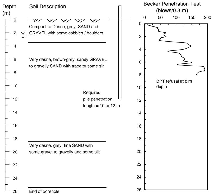
**Fig.2. Soil conditions and Becker Penetration Test results for Case History 1**
