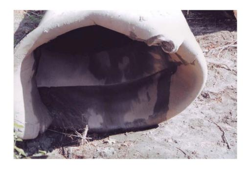
Fig. 4. Pile toe failure (d=1219 mm, t=12.7 mm), driven by D30-32 diesel hammer (Case History 1)
