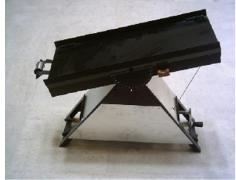
**Fig. 3.** Apparatus for measuring static coefficient of friction.
