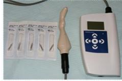
**Figure 6:** A photograph showing Osstell™ mentor measurement probe, power adapter and commercially available transducers.
