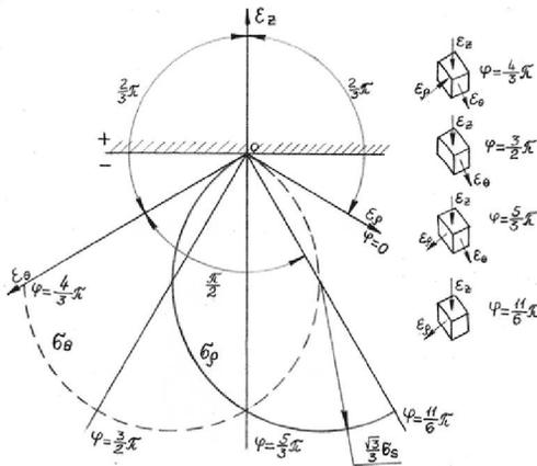
Fig.1. Stress state and strain types in flanging
