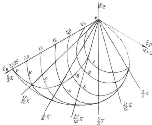
Fig. 3. Ways and distribution of deformations at the second stage of strain (curves 1 and 2-7 of strain distributions on initial and the subsequent stages of strain, directions  $4\pi/3 \dots 11\pi/6$  - ways of deformations, line 8 - line of the greatest circumferential strains.)
