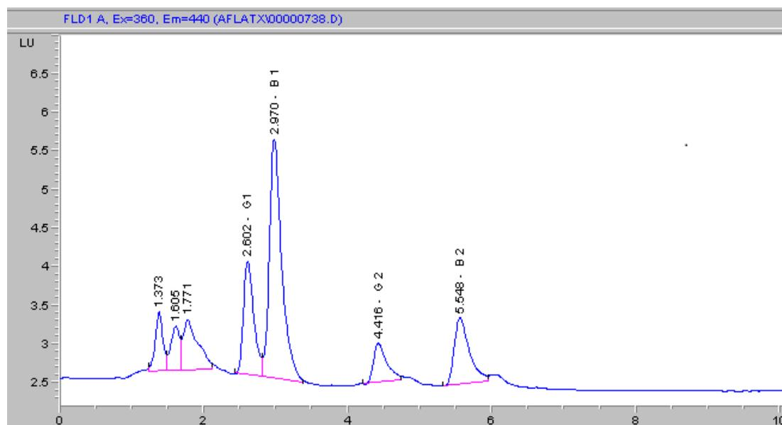
**Figure (2): High Performance Liquid Chromatogram of a standard of aflatoxins (AFG<sub>1</sub>, AFB<sub>1</sub>, AFG<sub>2</sub> and AFB<sub>2</sub>)**
