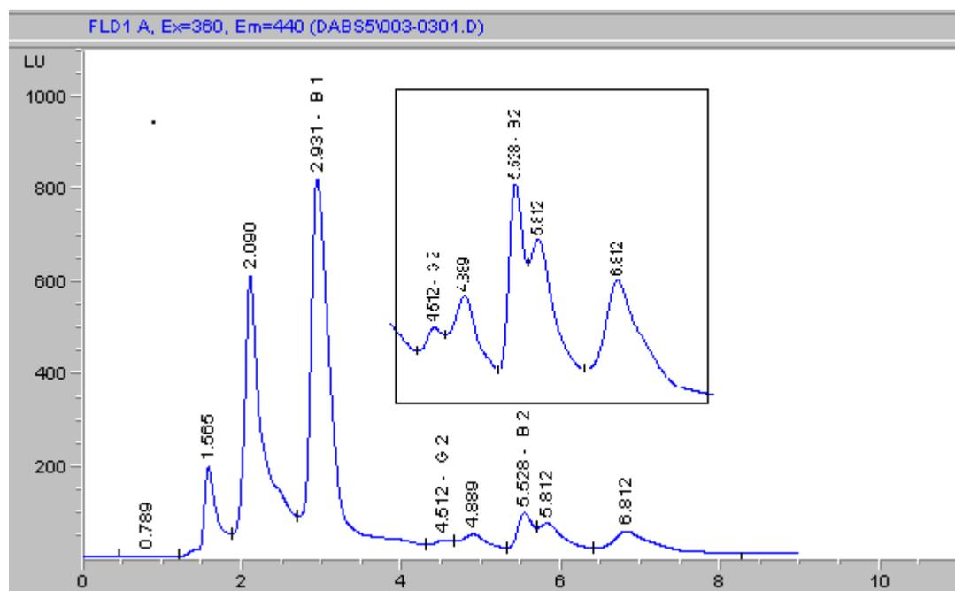
**Figure (1): High Performance Liquid Chromatogram of a positive sample of aflatoxins (AFG<sub>1</sub>, AFB<sub>1</sub>, AFG<sub>2</sub> and AFB<sub>2</sub>)**
