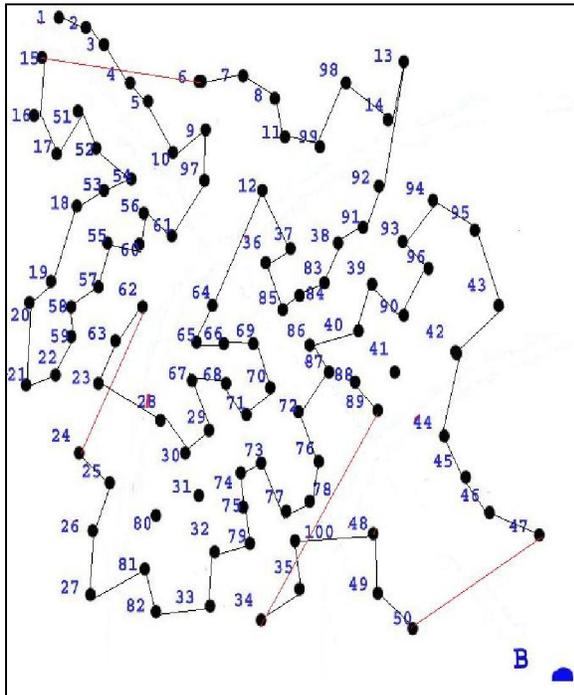
Figure 4. The PEGASIS chain construction phase with the simulation scenario
