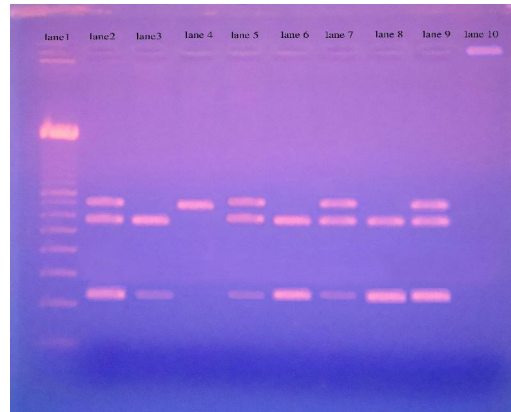
Figure (1): The three genotypes identified: lane 1 correspond to DNA (GeneRoler™ low range 25-700 bp) ladder; lane 2, 5, 7 and 9 correspond to GC genotype (58,140 and 198 bp); lane 3,6 and 8 correspond to GG genotype (58 and 140 bp) and lane 4 correspond to CC genotype (198 bp).
