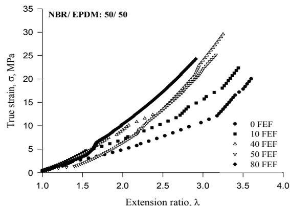
Fig. 3: Tensile stress- strain curves for NBR/ EPDM: 50/ 50 blend composites.
