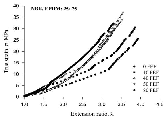
Fig. 4: Tensile stress- strain curves for NBR/ EPDM: 25/ 75 blend composites.
