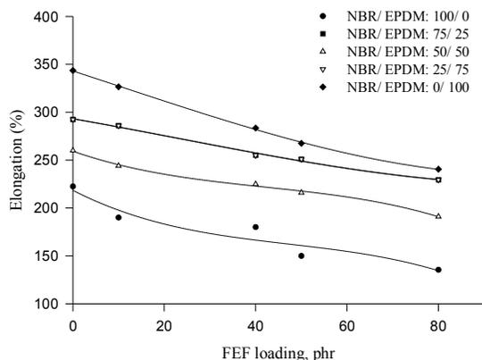
Fig. 7: Elongation at breaking point vs. filler loading for various blends.
