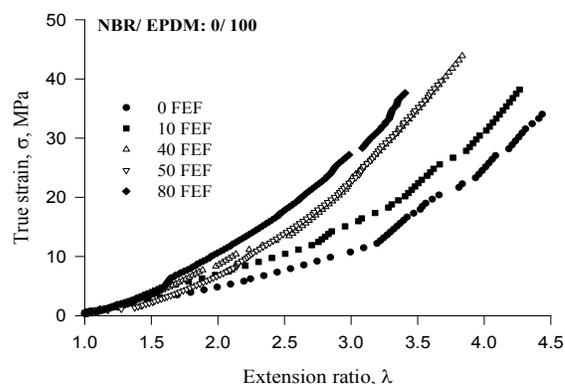
Fig. 5: Tensile stress- strain curves for FEF/ EPDM composites.
