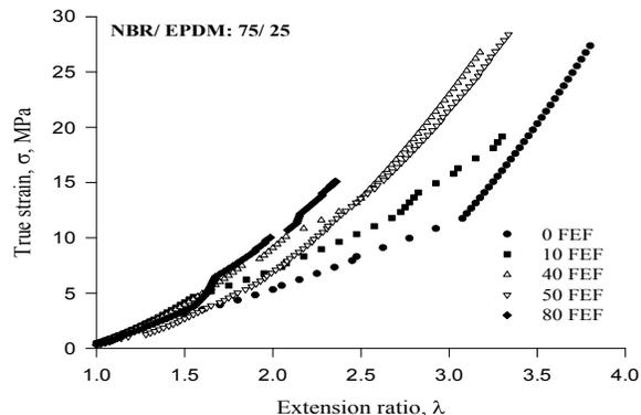
Fig. 2: Tensile stress- strain curves for NBR/ EPDM: 75/ 25 blend composites.
