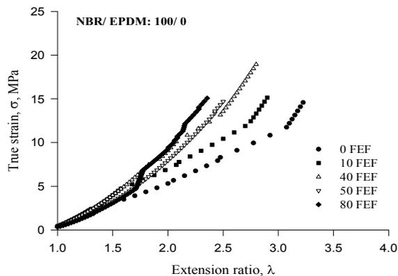
Fig. 1: Tensile stress- strain curves for FEF/ NBR composites
