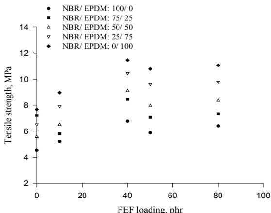
Fig. 6: The variation of tensile strength against filler loading for various blends.
