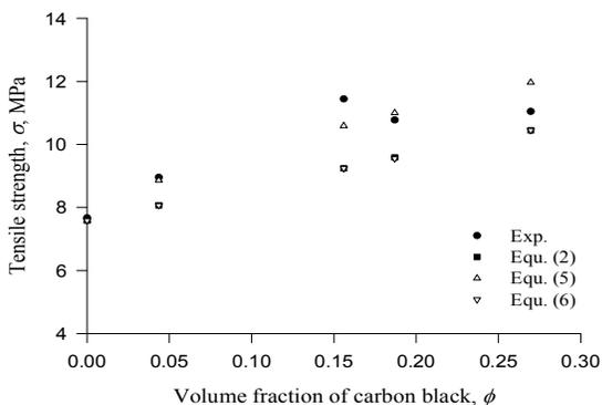
Fig. 8: Tensile strength vs. filler volume fraction fitted by difference models.
