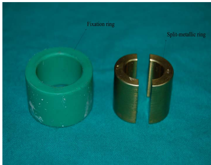
Figure (1): The fixation ring and the split-metallic ring used for the preparation of the specimens for measuring the “recovery from deformation”.
