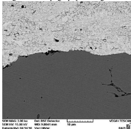
Fig.5: SEM micrograph of substrate-coating interface
