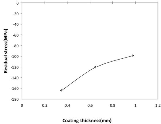
Fig.6: Compressive Residual stress from curvature method
